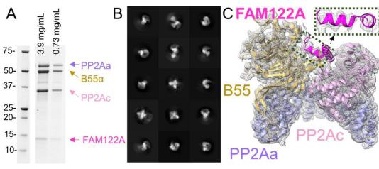
Fig. The PP2A:B55-FAM122A quadruple complex. A. SDS-PAGE gel of PP2A:B55 (PP2Aa/PP2Ac/B55; expressed in mammalian or E. coli cells; purified using purification steps) bound FAM122A stains (FAM122A. weakly). B. Representative 2D class averages of the PP2A:B55-FAM122A quadruple complex. C. Preliminary (small dataset) map fit with PP2A:B55 reveals the presence of density corresponding to FAM122A.
