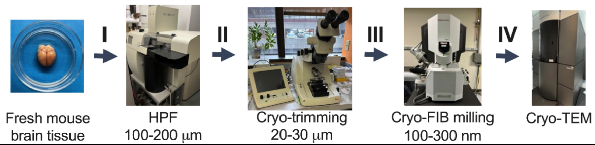
Figure 1. Workflow for preparation of fresh brain tissue for cryo-EM imaging. (I) 100-200 \mu\text{m} -thick sample of fresh mouse brain tissue is painted into a carrier. (II) Carrier is loaded into a high-pressure freezer (HPF) for immediate cryo-preservation. (III) The HPF sample is trimmed in a cryo-ultramicrotome to 20-30 \mu\text{m} thickness. (IV) The sample is thinned via cryo-FIB milling to a final 100-300 nm thickness, followed by imaging of the lamellae in a cryo-TEM.
