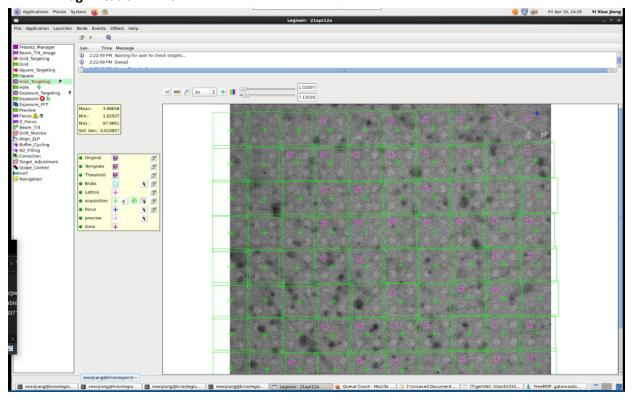
Pre-exposure at the "hole level"; these images allow us to see which holes have our fibril particles; then we perform manual target selection (green box) and focus selection (blue x); this pre-exposure beam is ~200x dimmer than the exposure beam and thus shouldn't damage sample
