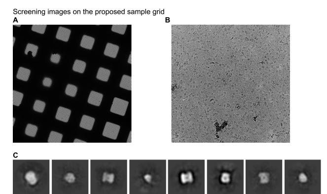
**A**, Atlas-level image on the sample grid. **B**, Data-level image on the sample grid. **C**, Representative 2D classes from screening images showing that target protein is well-behaving.
