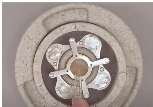
Figure 3. Ethane Holder Assembled. Proper ethane tip placement shown.
