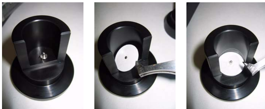
figure 1-21 Loading the filter paper disk and protective plastic backer
