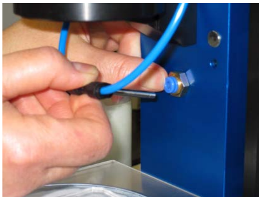
figure 1-42 Disconnect the pneumatic supply for the blotter assemblies
