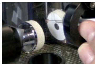
figure 1-31 Applying sample aliquot to the support film
