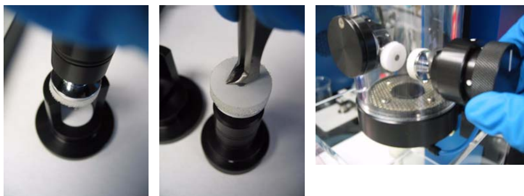
figure 1-22 Attaching the filter paper disk and inserting the blotter
