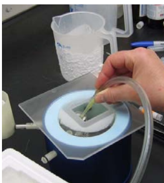
figure 1-25 Condensing ethane directly into the pre-cooled ethane pot
