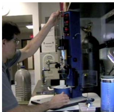
figure 1-30 Raising the plunge rod to full upward (firing) position
