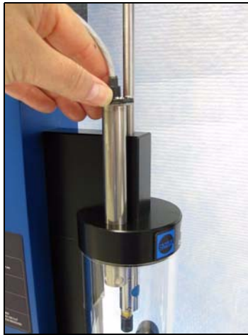
figure 1-12 Insertion of Omega temperature/humidity sensor
