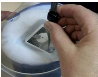
figure 1-37 Disconnect the black securing clip on the plunge tweezers to free the frozen hydrated grid
