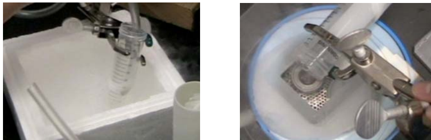
figure 1-26 Pre-cooling the conical tube and then pouring the condensed ethane into the pre-cooled ethane pot
