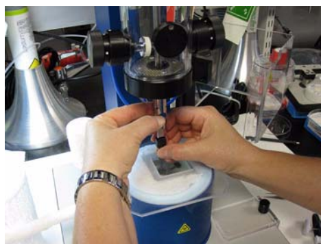
figure 1-34 Pressing the quick disconnect push button to release the plunge tweezers from the plunge rod
