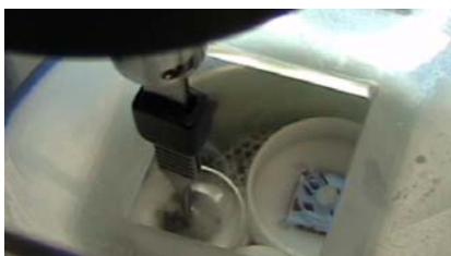
figure 1-33 Grid plunging into the liquid ethane
